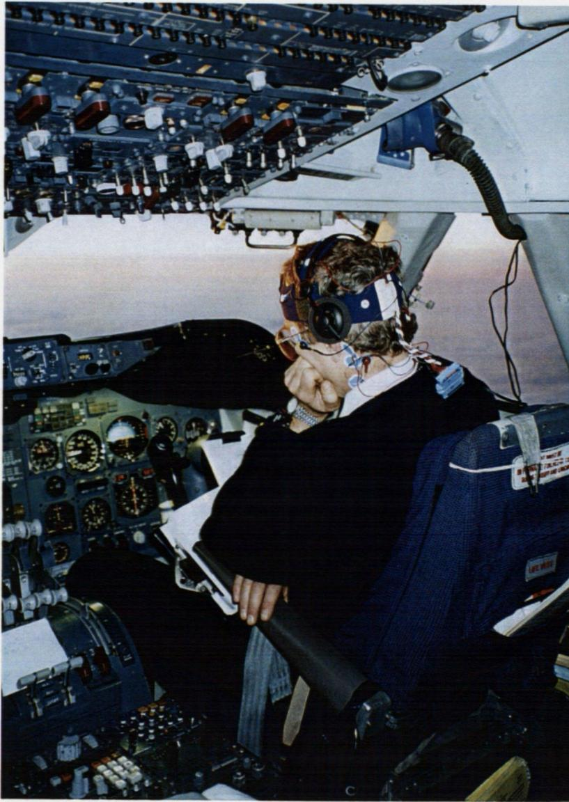
Figure 1 The pilot on the flight deck, showing the EEG, EOG and EMG electrodes in position. The left wrist actigraph is also visible
