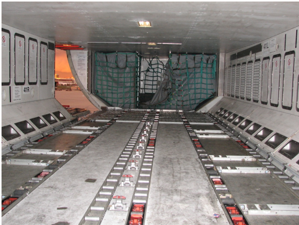
Figure 2: Typical A330 aft cargo hold (looking aft)
