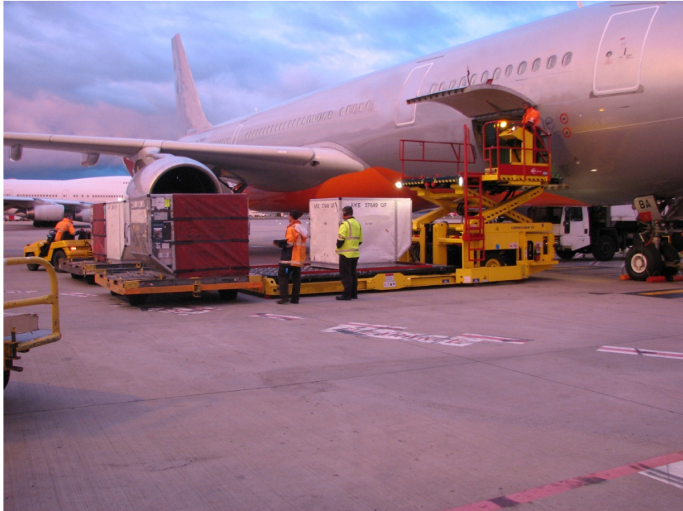
Figure 1: Typical AKE-type ULD loading into an A330 forward hold
