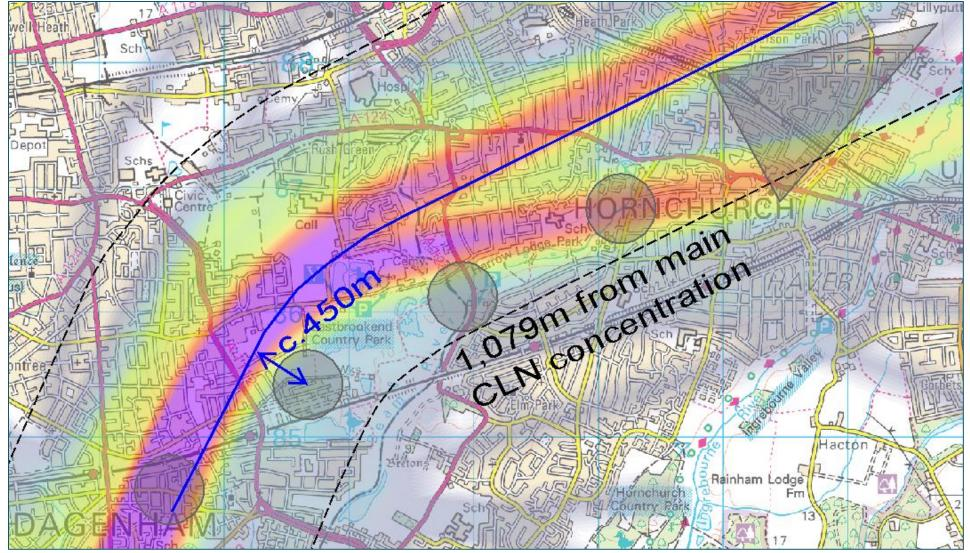
Example CLN SID vs predicted black-dot path vs CAP1498's definition of "overflight" using an elevation angle of 48.5°.
