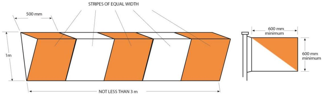
indicate the boundary of an area unfit for the movement of aircraft.
