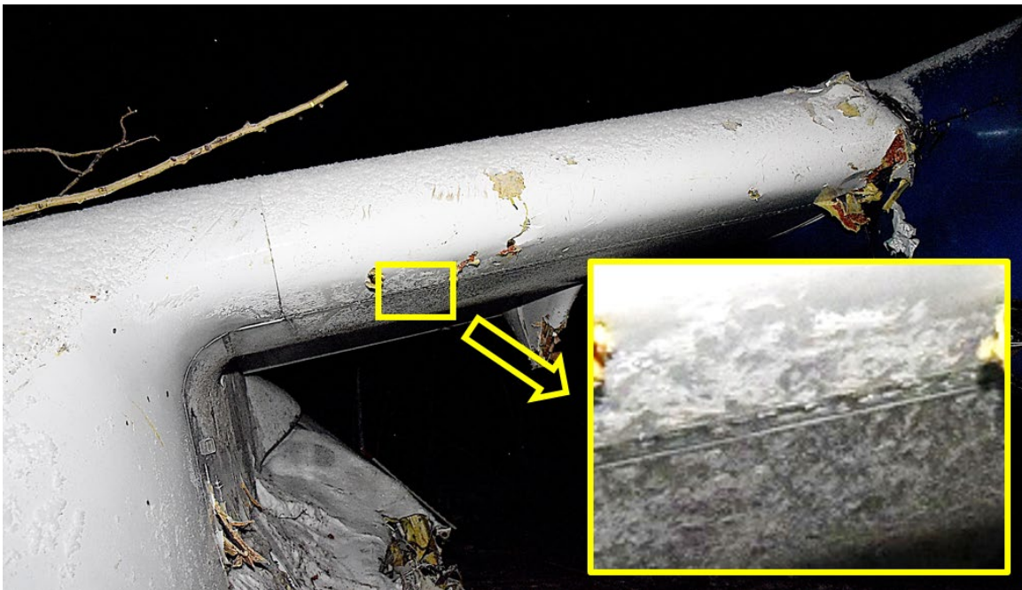
Figure 18. Photo of inner left wing with inset image showing surface contamination on lower leading edge (Source: Royal Canadian Mounted Police, with TSB annotations)
