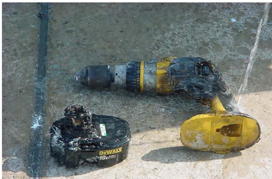
In this incident, the drill was activated, but the chuck could not rotate and so it overheated, resulting in a fire. Devices which can generate this type of heat if inadvertently activated must be carried in protective cases and, if possible, have trigger locks engaged.
