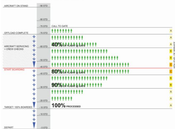
CODE E AIRCRAFT, BOEING 747-400, 3-CLASS, 90MIN TURN AIRCRAFT TURN-AROUND IDEAL BOARDING PROCESS
