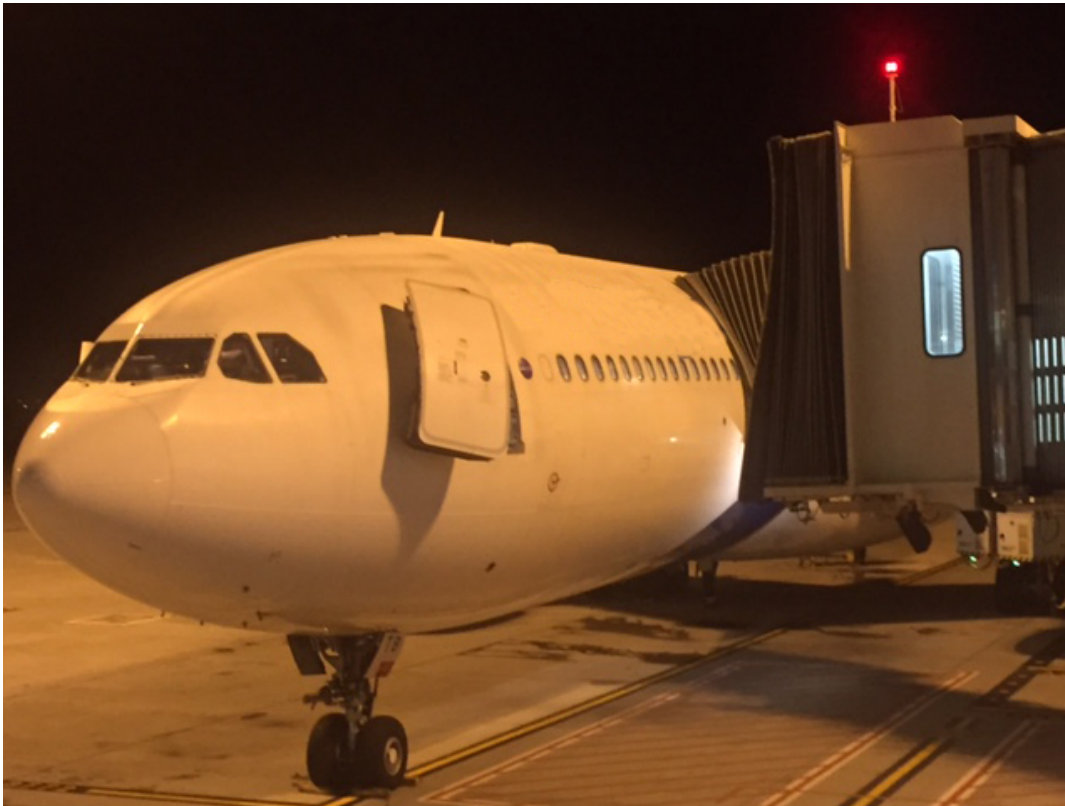
Figure 2: The aircraft’s forward fuselage showing the dislocated forward-left door. The slight indentation in the fuselage skin forward of the door is not visible. The aerobridge is shown retracted from its position when struck by the aircraft
